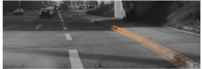
Fig. 1. A typical reconstruction result. The reconstructed curbstone is marked by red vertical lines, while the orange horizontal lines mark the attachment pieces of the neighboring surfaces.
