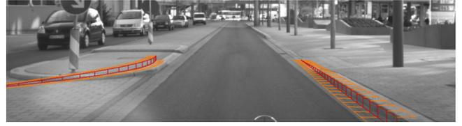
Fig. 8. Example showing the limitations of the utilized curb model. The assumptions are violated to much by the geometry of the traffic isle to allow a proper reconstruction.
