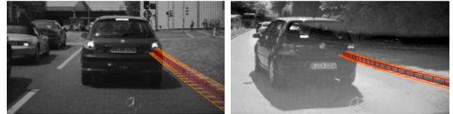
Fig. 2. Two examples for partial occluded curbs. The stabilizing cubic curb model provides a prediction of the curb’s characteristics in occluded regions.
