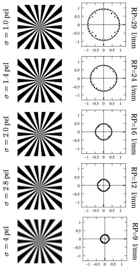
Figure 5: Siemens - star at various steps of image sharpness ( $\Delta x = 15 \mu\text{m}$ ,  $\sigma_n = 1gr$ ,  $\text{SNR} = 255$ ). left: test image, right: histogram of edges, resolving power of optimal edge detector.
