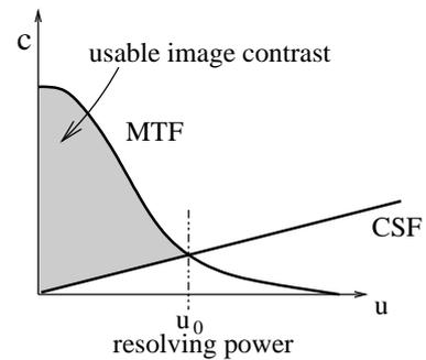
Figure 3: Relations between the modulation transfer function (MTF), the contrast sensitivity function (CSF) and the resolving power (RP).
