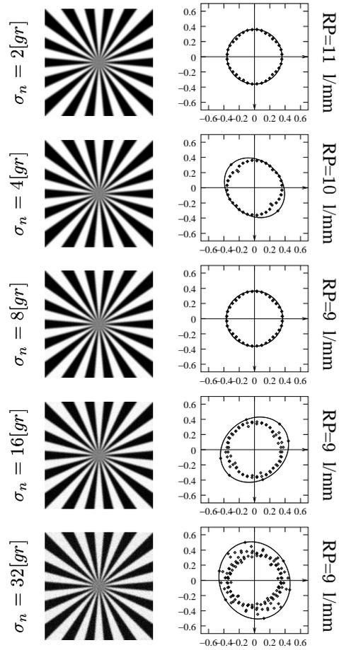
Figure 6: Siemens star with  $\sigma = 2.8 \text{ pel}$  at various steps of image noise ( $\text{SNR} = 128, 64, 32, 16, 8$ ).
