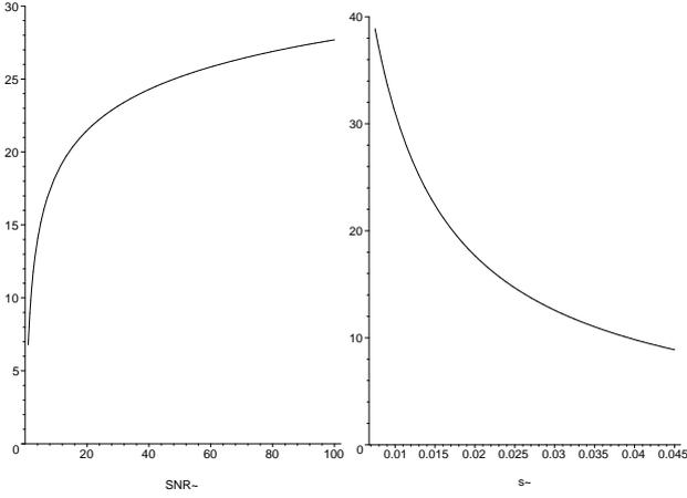
Figure 4: Resolving power in lines/mm for aerial images with a pixel size of  $15 \mu\text{m}$  as a function of SNR (left,  $\sigma = 1$ ) and of the width  $\sigma$  of the PSF (right, SNR=10)
