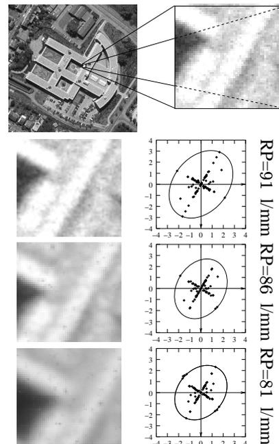
Figure 8: Aerial images with various image sharpness. Top: whole original image with image patch. Left: image patch at various steps of sharpness. Right: edge histogram, resolving power.
