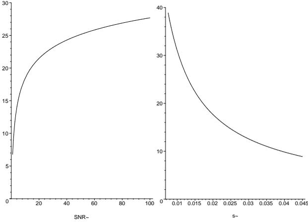
Figure 4: Resolving power in lines/mm for aerial images with a pixel size of  $15 \mu\text{m}$  as a function of SNR (left,  $\sigma = 1$ ) and of the width  $\sigma$  of the PSF (right, SNR=10)
