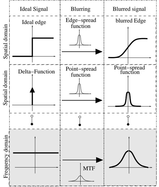
Figure 2: Edge spread function, point spread function and modulation transfer function.
