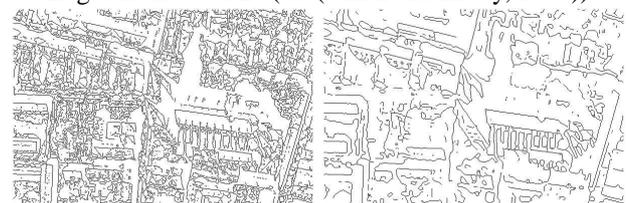
Figure 1: Effect of two different edge detectors on aerial images of different sharpness. The same parameters were taken for both images, no attempt was made to obtain the best results in all four cases.
