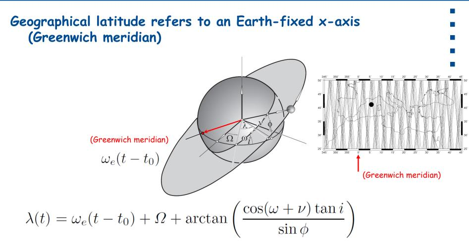
This means we have to add the Earth's rotation angle, to arrive at Earth-fixed longitude. (note Earth rotation is simplified here, assuming ω<sub>e</sub> = 2π / sidereal day)
