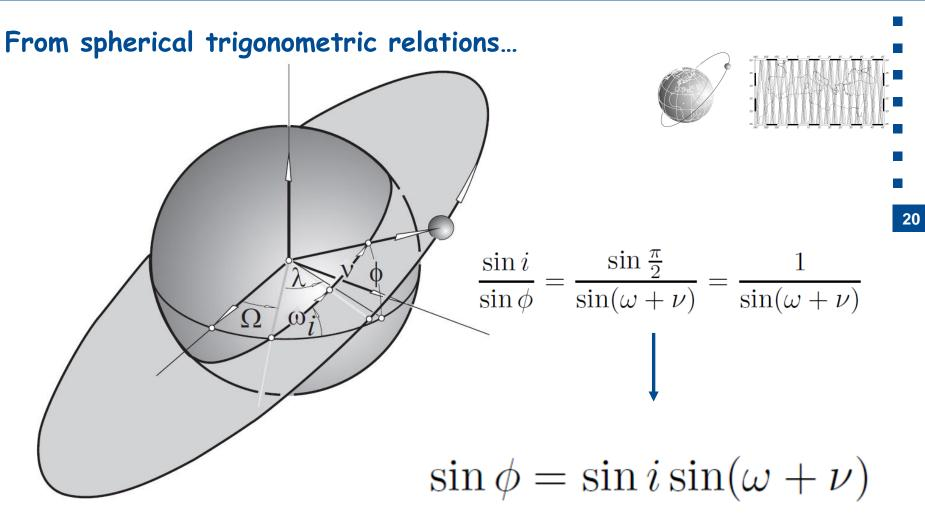
... we find the spherical latitude as a function of the mean anomaly, for given orbit inclination and argument of the perigee
