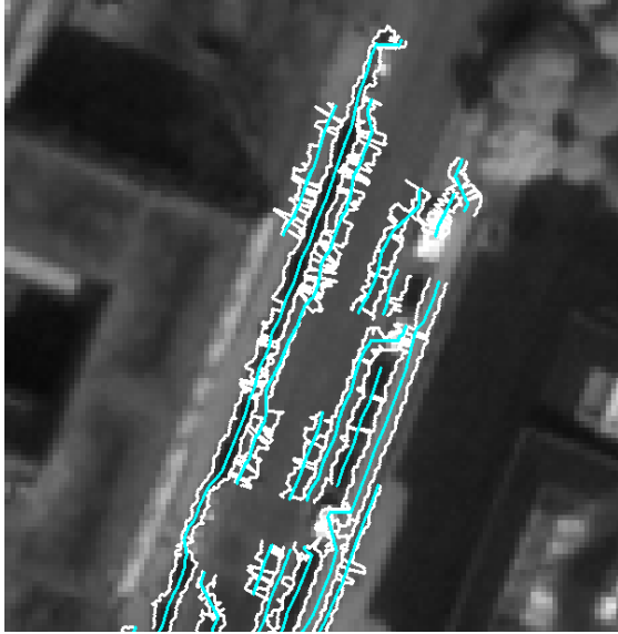
Figure 6: Extracted ribbons: medial axis (cyan) and width function (white).
