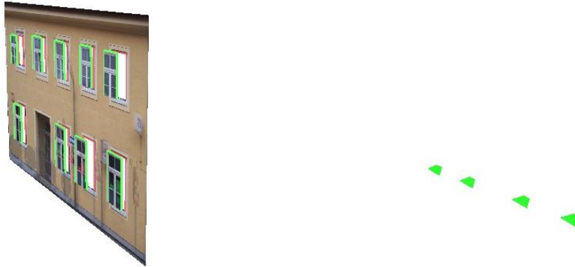
Figure 10. Bright building seen from the back – the windows are marked in red on the facade and in green behind the facade; cameras are given as green pyramids with the tip defining the projection center and the base the viewing direction
