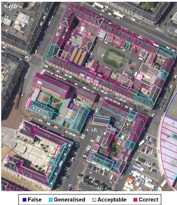
Figure 8: Manually labelled roof facets of the realistic dataset.
