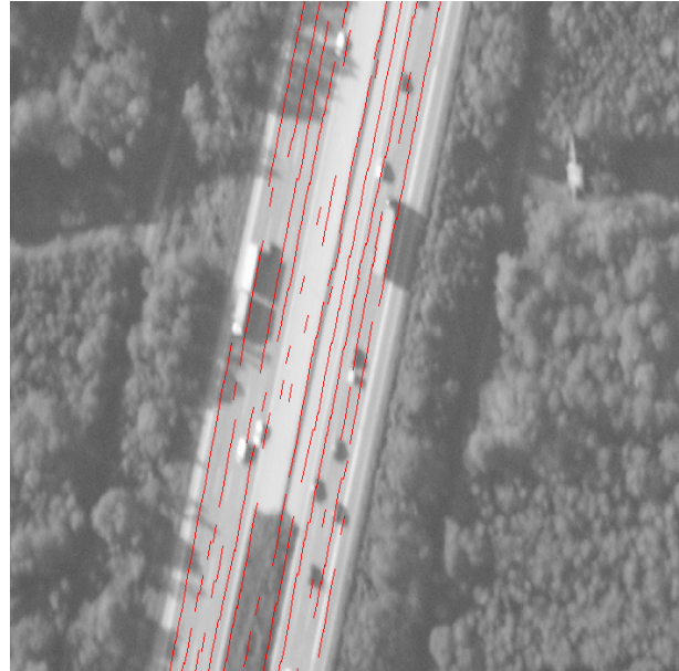
Figure 2. Intermediate result of lane extraction
