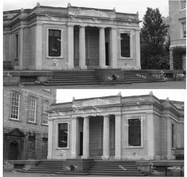
Figure 7: The 55 correspondences, which were automatically extracted using the Lowe region detector and used for the orientation procedure.
