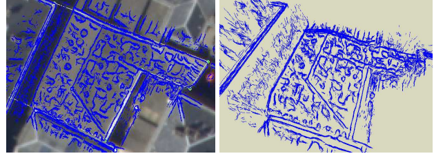
Figure 4: Reconstruction of edgels applied on an under-modelled facet. On the left, edgels projected on one image. On the right, a 3D view of the edgel set. The main structures of the roof building are well reconstructed wherever image contours have been extracted.
